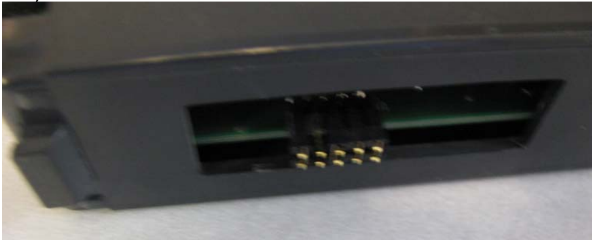
F4-08THM-n jumpers (Five pairs of pins unless it is a -1, -2, or -3 then there will only be three)
